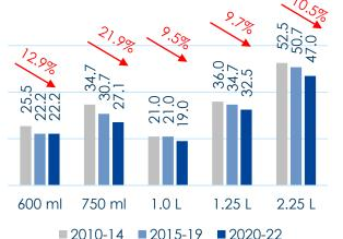
Plastic usage reduction through light weighting of Preforms and Closures for PET bottles. Phasewise implementation of certain SKUs is under process
